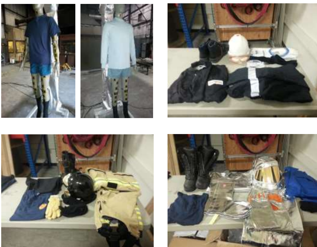
Figure 2 Clothing ensembles; upper left under garments, upper middle long sleeve undershirt, upper right operator's clothing, lower left firefighter's clothing, lower right aluminized clothing
